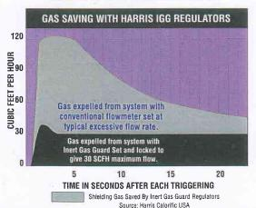
Conversely, the lower curve illustrates how Harris Sav 'T' Lock regulators can significantly reduce gas waste by reducing surge and delivering a controlled maximum flow rate.
